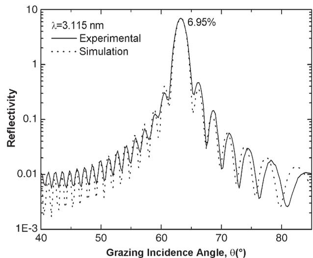
Fig. 5. Solid line: near normal-incidence soft X-ray reflectance measured at a wavelength of  $3.115\text{nm}$  showing a maximum of  $6.95\%$  at  $\theta=63.25^\circ$ . Dotted line: best fit IMD simulation of the reflectance. The simulation yielded a period of  $\Lambda=1.741\text{nm}$  and interface widths of  $\sigma=0.2\text{nm}$ .
