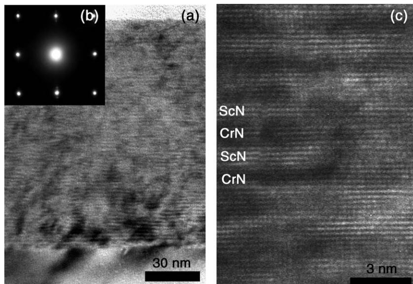
Fig. 3. Cross-sectional TEM micrograph from a CrN/ScN superlattice with the modulation period  $\Lambda$  of 1.7 nm and interface widths  $\sigma$  of 0.18 nm grown at  $735^\circ\text{C}$  with ion assisting energies  $E_{\text{Ion,CrN}}=24$  eV and  $E_{\text{Ion,ScN}}=28$  eV; (a) overview, (b) selected area electron diffraction pattern obtained along the MgO [010] zone axis, and (c) high-resolution image.
