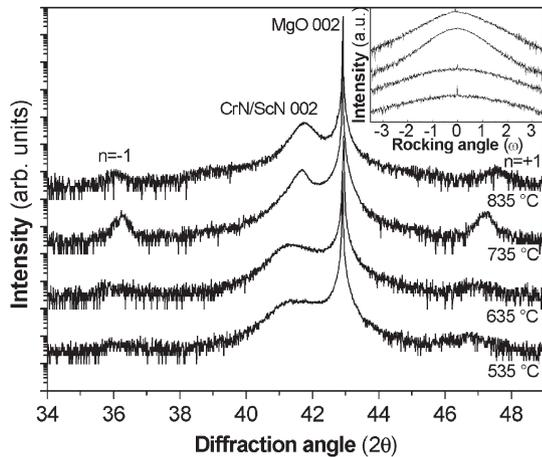
Fig. 1. Overview XRD  $\theta$ – $2\theta$  scans over the average CrN/ScN 002 Bragg peak as well as the first orders ( $n=\pm 1$ ) superlattice satellites from films synthesized at four different growth temperatures (535, 635, 735, and 835 °C) using a floating substrate potential. The inset shows the  $\omega$ -rocking curves over the Cr/ScN 002 peak for the same superlattices arranged in the same order as in the main figure.
