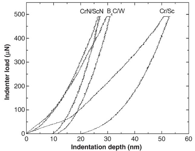
Fig. 7. Load–displacement curves from the nanoindentation experiments on 1  $\mu\text{m}$  thick epitaxial CrN/ScN superlattice films on MgO grown according to the optimal growth process determined in this work. As comparison, load–displacement curves for a 1  $\mu\text{m}$  thick state-of-the-art Cr/Sc X-ray multilayer mirror as well as a 0.34  $\mu\text{m}$  thick B<sub>4</sub>C/W X-ray multilayer mirror, both on monocrystalline Si-substrates.
