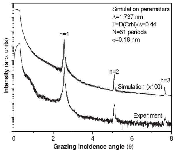
Fig. 2. Hard X-ray reflectivity (HXR) scans from an epitaxial (002) oriented CrN/ScN superlattice film grown at  $T_S=735\text{ °C}$  on MgO(001) substrate with ion assistance energies of  $E_{\text{Ion,CrN}}=24$  and  $E_{\text{Ion,ScN}}=28\text{ eV}$  (lower curve) and simulated HXR (top curve).
