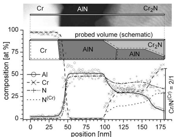
Fig. 5. EDX line scan at an  $\text{Al}_{0.7}\text{Cr}_{0.3}\text{N}$  sample annealed at  $1450\text{ }^\circ\text{C}$ . Fitted curves for Al, Cr, and N are provided.  $\text{N}^{(\text{Cr})}$  shows N bonded to Cr. The schematic drawing indicates the probed volume under the line scan.
