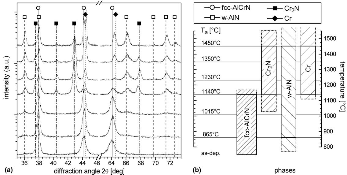
Fig. 2. (a) XRD evolution of an  $\text{Al}_{0.7}\text{Cr}_{0.3}\text{N}$  film with annealing temperature; (b) bars represent detected phases, dashed extensions indicate the estimated existence range of the phases that occur.
