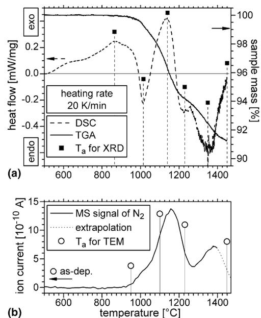
Fig. 1. (a) DSC and TGA of  $\text{Al}_{0.7}\text{Cr}_{0.3}\text{N}$  in inert atmosphere with indicated annealing temperatures for XRD measurements; (b) corresponding MS signal with marked temperatures for TEM investigations.
