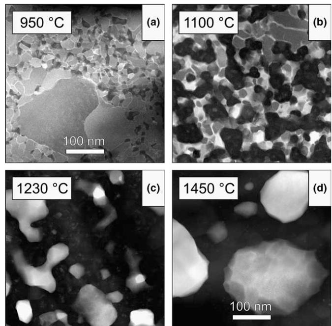
Fig. 4. STEM plan-view images (HAADF) of Al<sub>0.7</sub>Cr<sub>0.3</sub>N after annealing at (a) 950 °C; (b) 1100 °C; (c) 1230 °C; (d) 1450 °C.
