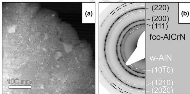
Fig. 3. (a) STEM plan-view image (HAADF) of  $\text{Al}_{0.7}\text{Cr}_{0.3}\text{N}$  in the as-deposited state; grains appear in a uniform grey tone, a thickness induced contrast-gradient is superposed; (b) SAED pattern with standard diffraction rings for fcc-AlCrN and w-AlN.
