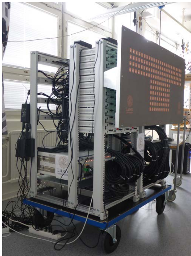
The LU Massive MIMO testbed LuMaMi.
